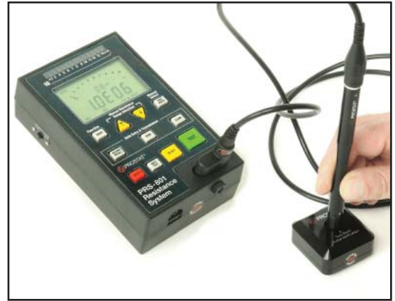
Figure 8: Insert PRF-912B Fixture into PRV-913B Verifier and Measure Verifier Resistance
