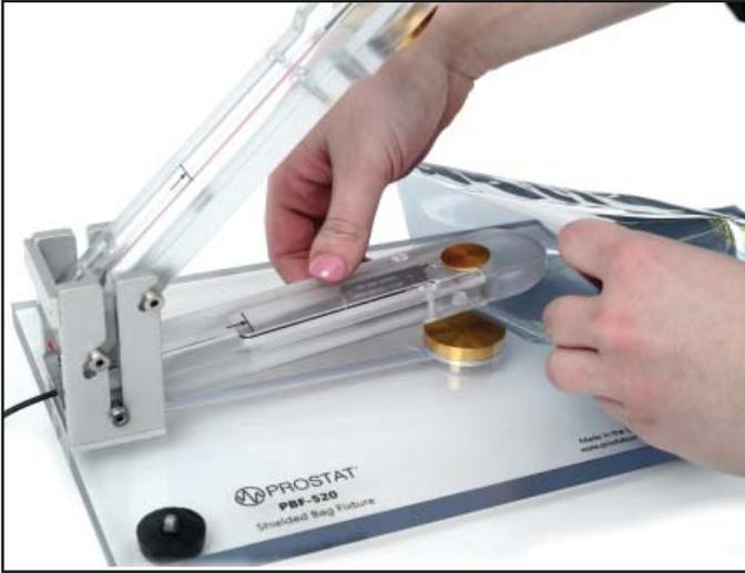
Figure 10: The Capacitive Arm inside the shielded bag.
