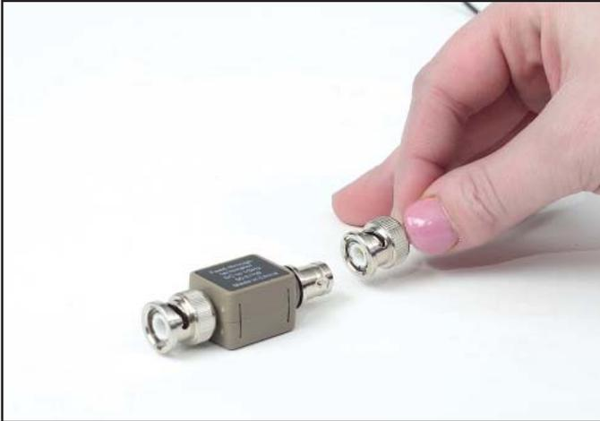
Figure 5: The 50 ohm terminator connects to the current probe.
