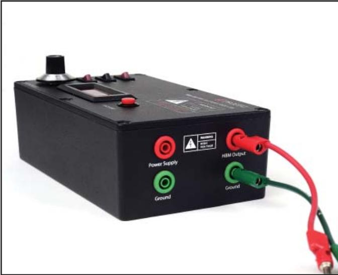
**Figure 1: Connect the short red lead to the HBM Output connector on the PDS-510**
